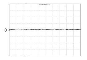
**Figure 12:** Input reflected ripple current, i<sub>s</sub>, through a 12µH source inductor at nominal input voltage and rated load current (20 mA/div, 1us/div)
