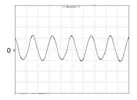
**Figure 14:** Output voltage ripple at nominal input voltage and rated load current (lo=full load)(50 mV/div, 1us/div) Load capacitance:  $1\mu$ F ceramic capacitor and  $10\mu$ F tantalum capacitor. Bandwidth: 20 MHz. Scope measurements should be made using a BNC cable (length shorter than 20 inches). Position the load between 51 mm to 76 mm (2 inches to 3 inches) from the module.
