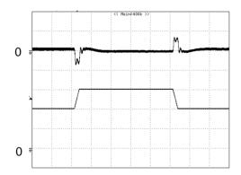
**Figure 8:** Output voltage response to step-change in load current (75%-50%-75% of lo, max; di/dt = 0.1A/µs). Load cap:  $10\mu$ F tantalum capacitor and  $1\mu$ F ceramic capacitor. Top Trace: Vout (100mV/div, 200us/div), Bottom Trace: lout (5A/div). Scope measurement should be made using a BNC cable (length shorter than 20 inches). Position the load between 51 mm to 76 mm (2 inches to 3 inches) from the module
