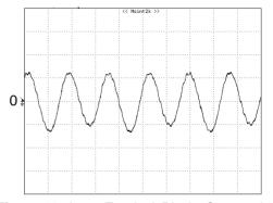
**Figure 11:** Input Terminal Ripple Current,  $i_c$ , at full rated output current and nominal input voltage with 12µH source impedance and 33µF electrolytic capacitor (100 mA/div, 1us/div)
