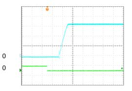
**Figure 5:** Turn-on transient at zero load current (10 ms/div). Vin=48V. Top Trace: Vout: 1.5V/div, Bottom Trace: ON/OFF input, 5V/div
