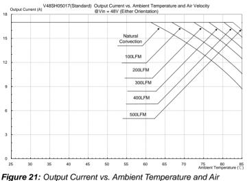
Velocity @ Vin=48V (Either Orientation, without heat spreader)
