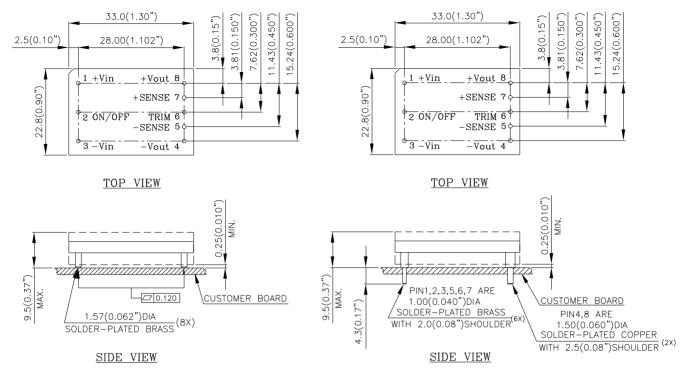
NOTES: DIMENSIONS ARE IN MILLIMETERS AND (INCHES) TOLERANCES: X.Xmm±0.5mm(X.XX in.±0.02 in.) X.XXmm±0.25mm(X.XXX in.±0.010 in.)
