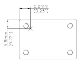
**Figure 22:** Temperature measurement location The allowed maximum hot spot temperature is defined at 110 °C.
