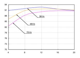
Figure 1: Efficiency vs. load current for minimum, nominal, and maximum input voltage at  $25^{\circ}$ C
