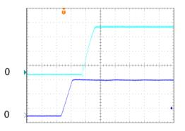
*Figure 7:* Turn-on transient at zero load current (10 ms/div). Vin=48V. Top Trace: Vout, 1.5V/div; Bottom Trace: Vin. 20V/div
