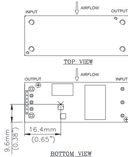
**Figure 17: Hot spot 1 temperature measurement location**
