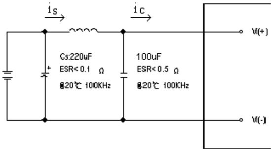
**Figure 8: Test Setup Diagram for Input Ripple Current**
