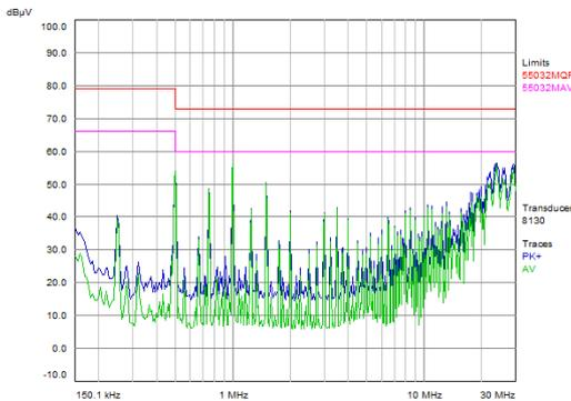
**Figure 12-2: Test Result of EMC (Vin=48V, Io=37.5A).**
