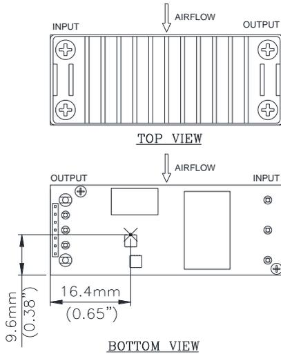
**Figure 19: Hot spot 2 temperature measurement location**
