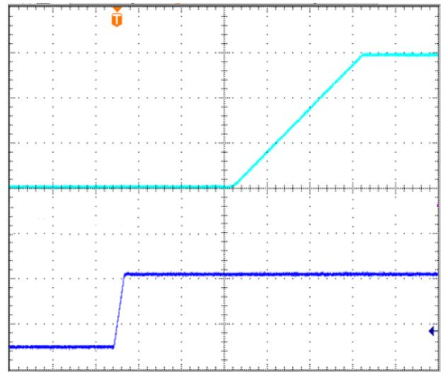
**Figure 5: Input Voltage Start-up at full load**
