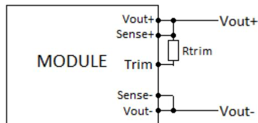
**Figure 15: Circuit configuration for trim-up (increase output voltage)**
