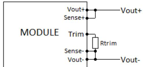
**Figure 14: Circuit configuration for trim-down (decrease output voltage)**
