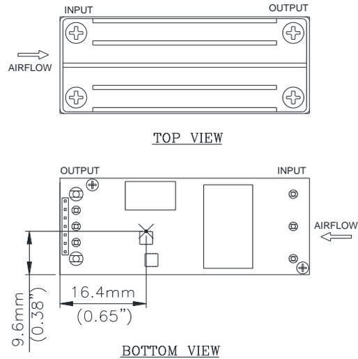
**Figure 21: Hot spot 3 temperature measurement location**
