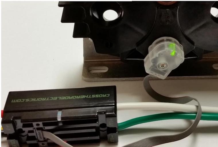
Note – Image shows a CTRE Mag Encoder, however CANCoder also displays color LED indicating magnet field strength.
