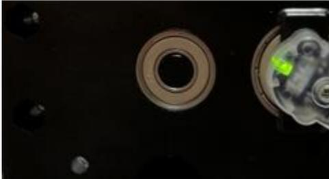
Note – Image shows a CTRE Mag Encoder, however CANCoder also displays color LED indicating magnet field strength.
