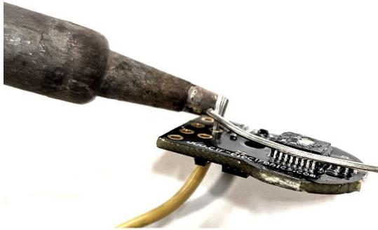
Tin the exposed portion of the wire-lead, until solder hole completely fills with solder. Cut the excess lead with diagonal cutters.
