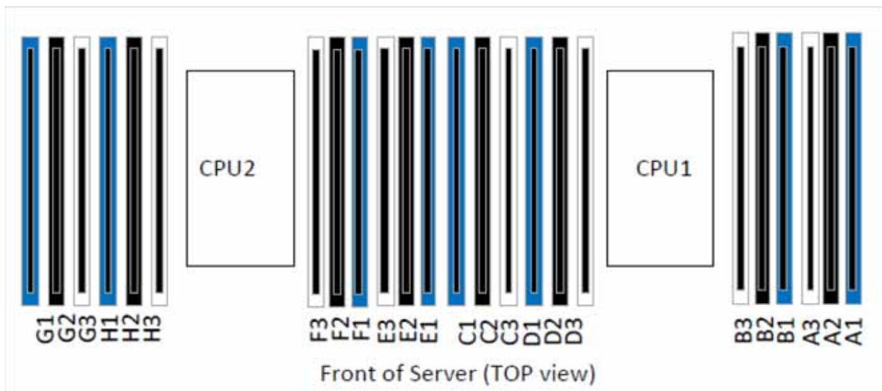
Figure 9 Physical Layout of CPU DIMM Channels and Slots
