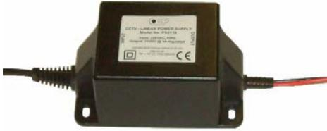
Designed as a power supply for single CCTV internal cameras although suitable for a wide range of other applications. The circuit is encapsulated in a black ABS case with an un-terminated input and output cable of 1 metre in length. Thermal protection is provided with a single shot fuse.
