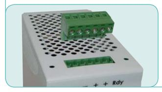
The 24VDC Output devices have 2 terminals, identified by RDY, that provide an external electrical indication of the power status. In case of failure: low output voltage or no output, the internal contact opens indicating to remote devices the abnormal situation. The 5W, 10W and 18W devices do not offer this unique feature, whereas all the others SPDs do.
