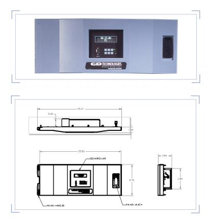
The Sageon<sup>®</sup> Plant Controller is a control and supervisory unit designed to control up to 225 parallel connected Sageon rectifiers (rectifier), and up to four parallel connected battery strings (standard configuration) in a 24VDC or 48VDC uninterruptible power system. It can be expanded to accommodate monitoring functions such as battery cell voltage, AC supply parameter, and site monitoring.
