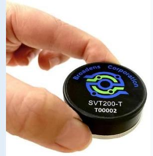
SVT200-T measures temperature and sends out the result every 15 seconds (measurement interval customizable), which has the fastest temperature update intervals among wireless sensors in the industry.
