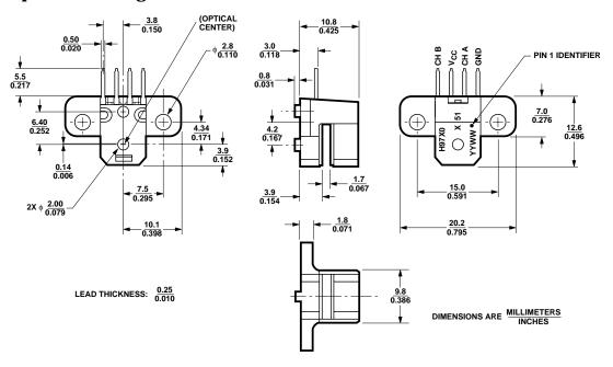
**Mounting Option #51 - Screwmount (Baseplane Mounting)**
