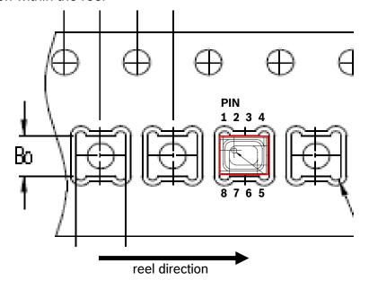
Figure 22: Orientation within tape
