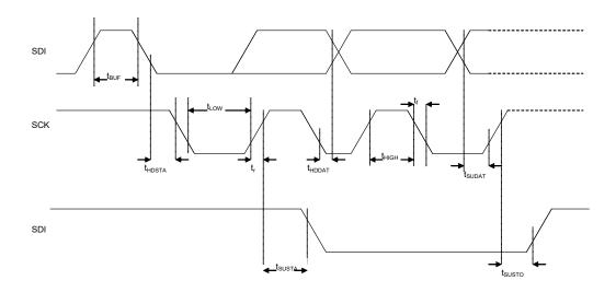
Figure 12: I<sup>2</sup>C timing diagram
