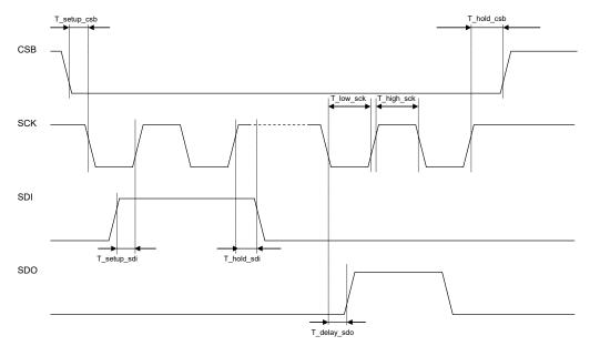
Figure 13: SPI timing diagram
