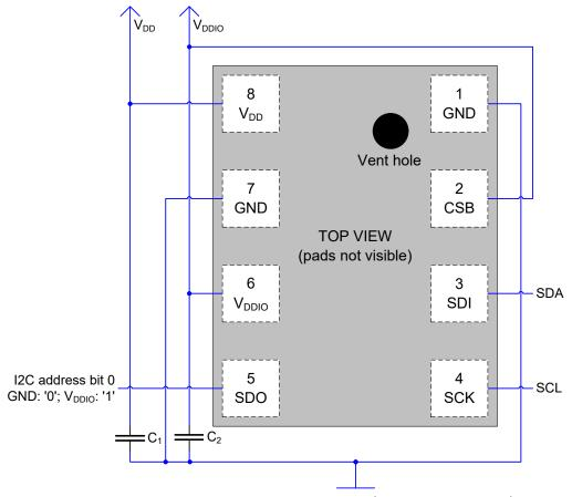
Figure 17: I<sup>2</sup>C connection diagram (Pin1 marking indicated)
