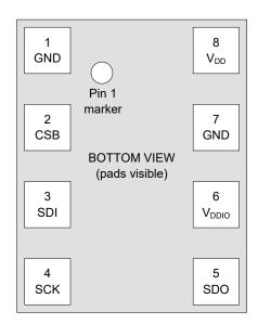
Figure 14: Pin-out top and bottom view
