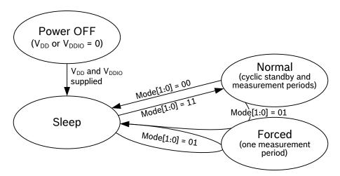
Figure 5: Mode transition diagram
