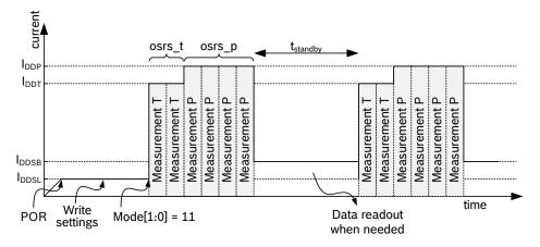
Figure 4: Normal mode timing diagram
