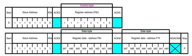
Figure 8: I2C multiple byte read
