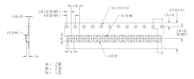
Figure 21: Tape and Reel dimensions
