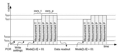
Figure 3: Forced mode timing diagram
