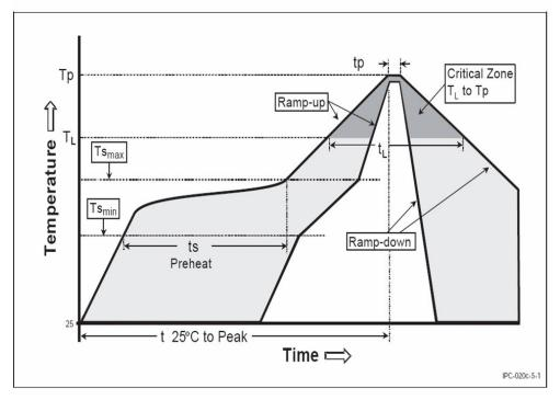
Figure 20: Soldering profile
