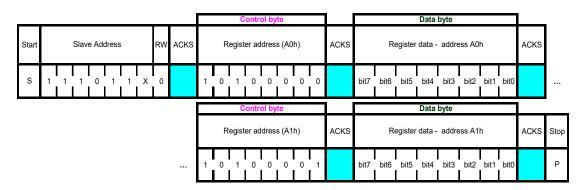
Figure 7: I<sup>2</sup>C multiple byte write (not auto-incremented)
