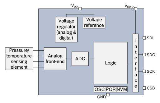
Figure 1: Block diagram of BMP280
