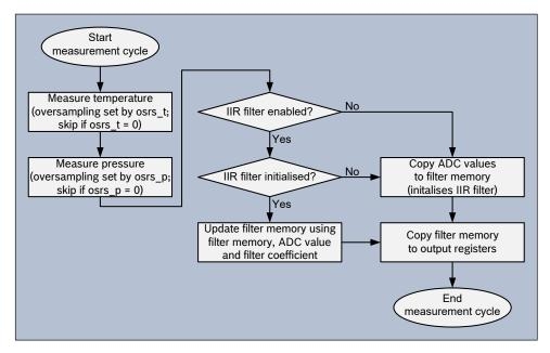
Figure 2: BMP280 measurement cycle
