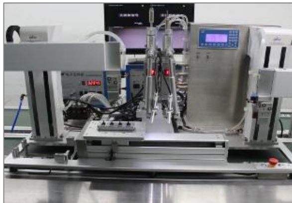
The micro welding robot with machine vision
