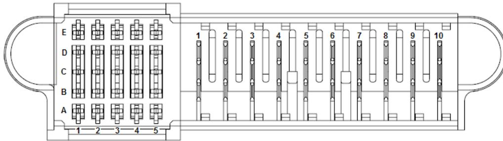
**Power Supply Connector:** Tyco Electronics P/N 1926736-3 or FCI connector 10133129-002LF or equivalent
