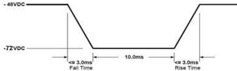
Figure 3. Minus 72 VDC Line Transient Test
