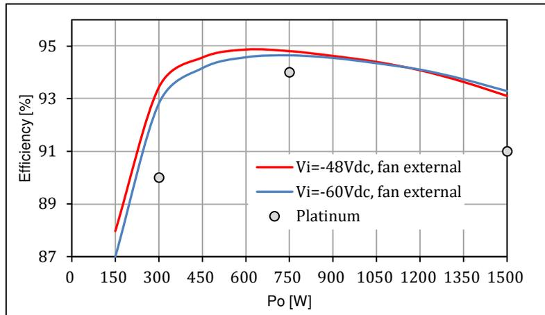
Figure 2. Efficiency vs. Load current (ratio metric loading)
