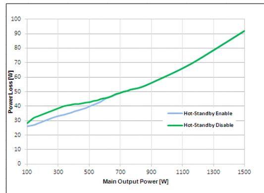
Figure 16. PSU power losses with/without hot-standby mode
