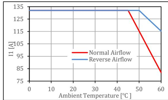
Figure 8. OCP Derating Curve with Ambient Temperature
