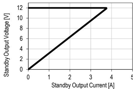
Figure 10. Current Limitation on 12 V<sub>SB</sub>
