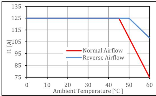
Figure 7. Iout Derating Curve with Ambient Temperature
