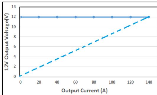
Figure 6. Current Limitation on  $V_1$
