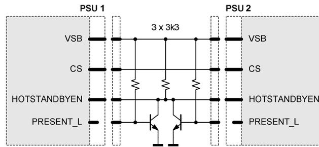
Figure 17. Recommended hot-standby configuration
