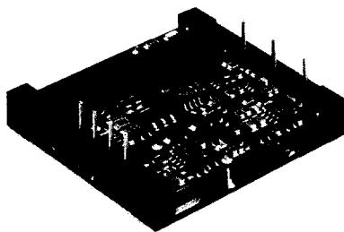
Input voltage range up to 75 V DC
