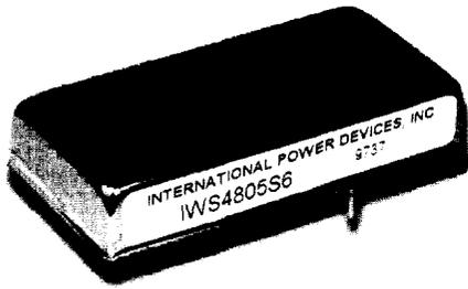
The IWS series converters offer excellent regulation and isolation in the industry standard 1 x 2 package. Available in several input versions, the IWS is perfect for industrial, datacom, or telecom applications. The IWS features shortcircuit protection, and 500VDC of isolation. Several output voltages are available, please see the IWD series for dual output applications.
