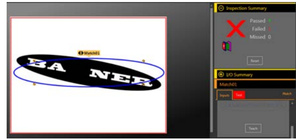
Figure 243. Bad Part—Missing Letter
