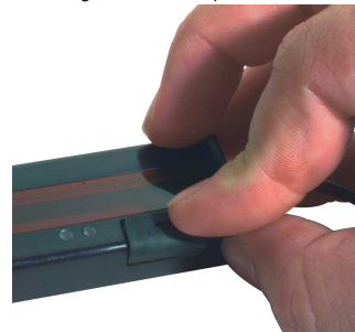
Figure 7. Cover Replacement – Pressing Cover
