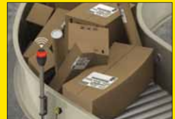
Manufacturing Line Blockage Indication A red, audible domed light alerts operators of congestion due to a box pile up.
