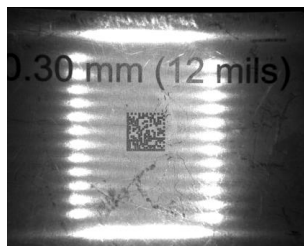
Figure 284. Multicolored DPM - Peripheral Group ALL Sectors On: Suboptimal Illumination
