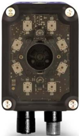
Figure 239. 1.3 MP Model with 8-LED Polarized Illuminator
