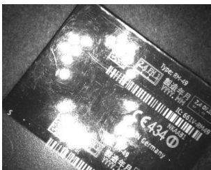
Figure 244. Example A: Incorrect Illumination
