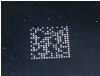
Figure 230. Directly Marked Dot Matrix Code Characterized by Outstanding Separation Distance between Adjacent Code Elements
