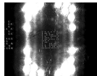
Figure 277. Multicolored DPM - Central Group: Incorrect Illumination
