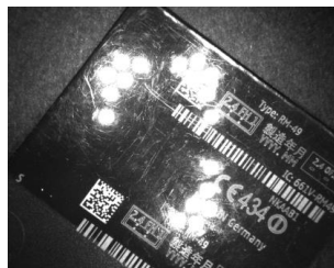
Figure 245. Example B: Good Illumination on Left Code
