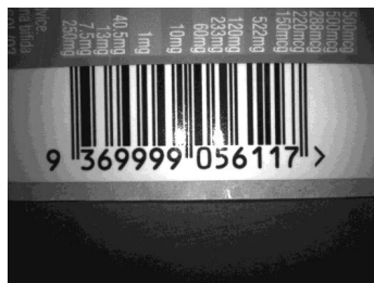
Figure 195. 1.2 MP Polarizer Model Reading Reflective Label
