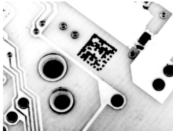
Figure 194. Data Matrix Code Directly Marked on PCB Surface by Using Laser Etching Technology
