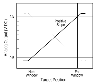
Slope—Voltage-Sourcing Models, 0.5 V to 4.5 V
