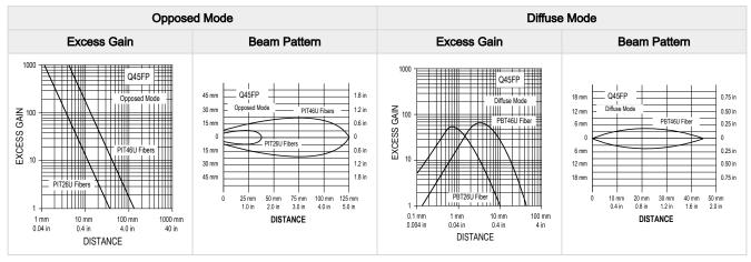
Plastic fiber diffuse mode performance curves are based on a 90% reflectance white test card.
