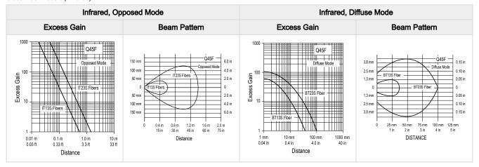
Glass fiber diffuse mode performance curves are based on a 90% reflectance white test card.
