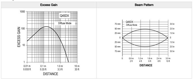
Diffuse mode performance curves are based on a 90% reflectance white test card.
