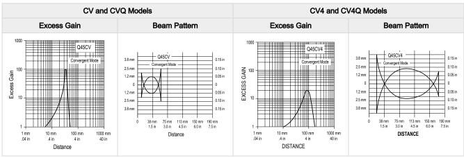
Convergent mode performance curves are based on a 90% reflectance white test card.
