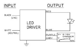
Maximum Wiring Distance (at full load) is 18AWG/18Feet
