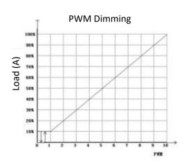
Notes: Dimming accuracy is ±10%lo Dimming load is <1mA, @10V
