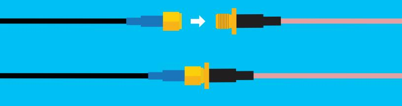
If you need to water proof a SMA connection, we highly recommend using a product like **Coax-Seal** to safely cover and prevent any water damage that may occur.
