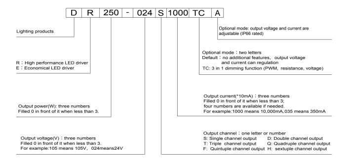
For example: DR250-024S1000TC means it is a high performance LED driver, output power 250W, output voltage 24Vdc, output current 10000mA, single output, with 3 in 1 dimming function.
