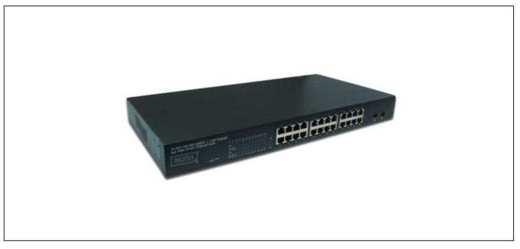
DIGITUS Web Smart Gigabit Ethernet PoE+ Switch 24-port RJ45, 2-port SFP, Half Powered, IPv6 Rack Mount, 195W
