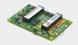
The AGQ300-48S1V2 series quarter-brick isolated DC-DC converter produces a single fully regulated output voltage of 1.2 Vdc. Rated at 72 watts, the converter can deliver up to 60 amps output current. It has a wide 2:1 input range of 36 to 75 Vdc and is designed primarily for use with standard 48 V telecommunications equipment supplies.
