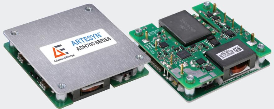
Advanced Energy's Artesyn ADH700 series half-brick isolated DC-DC converter provides a single regulated low noise output. ADH700-48S28 with 28V/25A output. It has a telecom input range of 36 to 65Vdc and is designed primarily for use with standard 48 V telecommunications equipment supplies. The converter's main application area is in low power and remote radio head (RRH) telecommunications applications.
