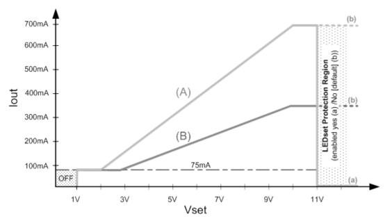
Case A:  $I_{max}$  =700mA, CLM disabled, 3DIM Module = 100% Case B:  $I_{max}$  =350mA, CLM disabled, 3DIM Module = 100%
