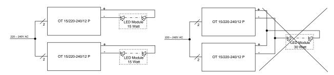
Power supplies can be connected in parallel on the primary side, but not on the secondary side
