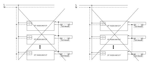
The installation of two or more OPTOTRONIC® OT 15/220-240/12 P Power supplies with common "-" or "+" wiring is forbidden.
