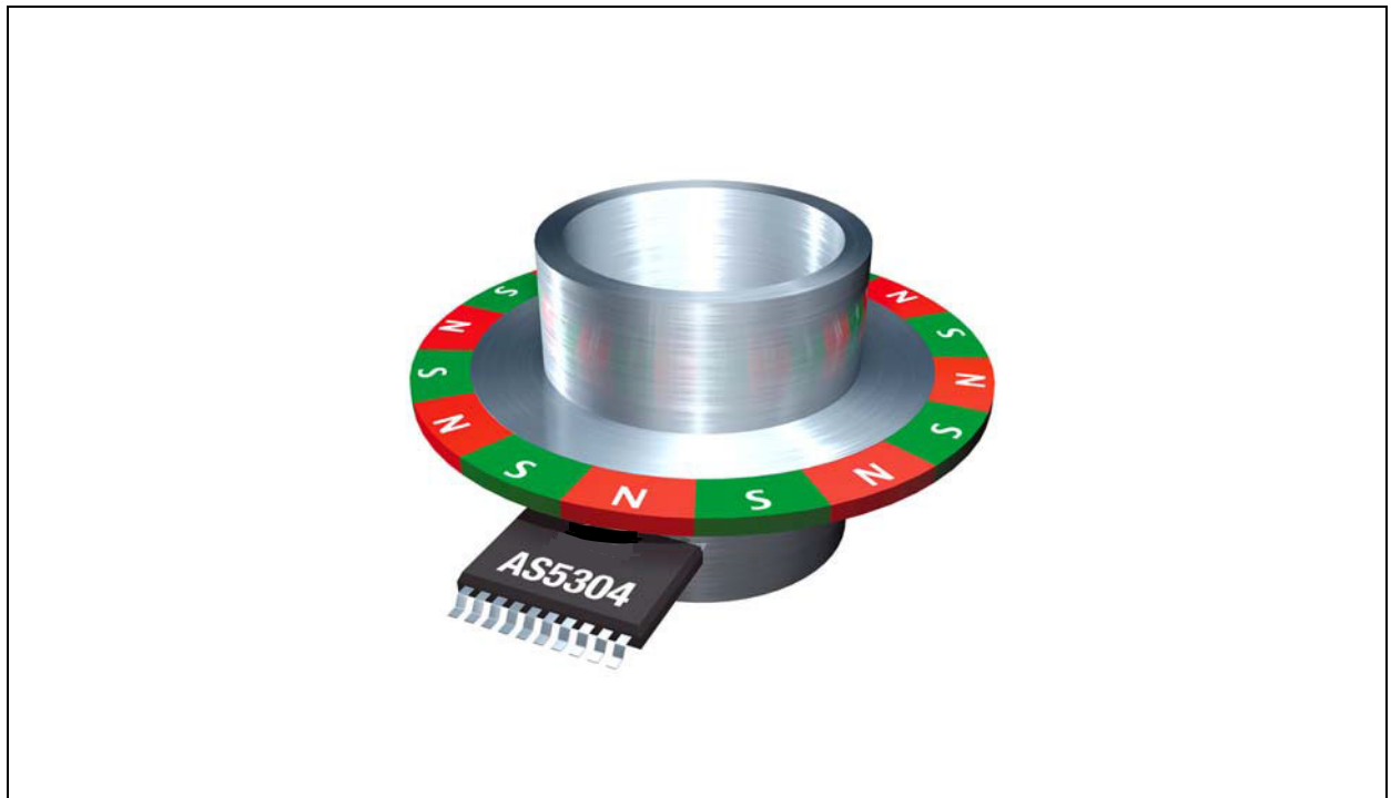
Figure 20: AS5304 (AS5306) with Multi-Pole Ring Magnet
