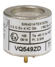
If a flammable gas is present when the bead is heated to about 400 to 500 °C, the gas will oxidise and the resultant release of energy will heat the bead still further. This increase in temperature is detected as an increase in resistance of the coil.
