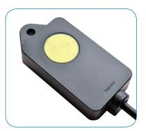
Designed to meet the needs of OEM manufacturers for low cost Carbon Dioxide (CO<sub>2</sub>) sensor installations, the Telaire T3022 Series provides reliable and convenient CO<sub>2</sub> measurement in an IP65-rated enclosure. Compatible with other sensors in the Amphenol Advanced Sensors product portfolio, the T3022 easily integrates into environmental monitoring and control systems via  $I^2C$  serial communication protocols.
