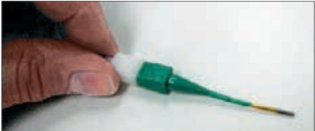
Plastic tool with contact in proper position.
