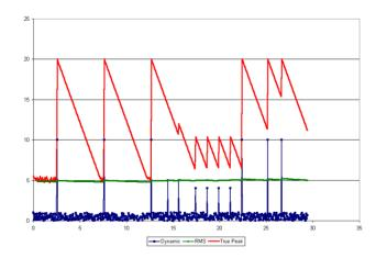
It then ramped back down over a time period of almost 5 seconds. During this "ramp down" the PLC/DCS has multiple opportunities to sample the signal and record the transient event.
