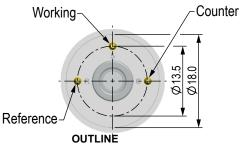
All dimensions are in mm All tolerances are ±0.2mm
