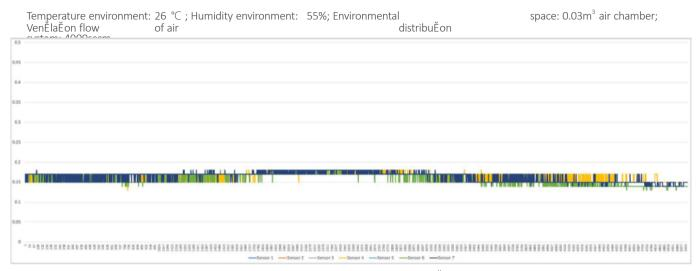
Test result: 12 hours clean air test, zero dril <0.2ppm (0-2ppm is the normal zero fluctua
