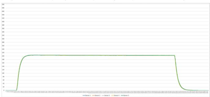
Test result: 2 hours venĚlaĚon, range dril <2ppm; (500ppm ±2% of full scale is the normal range);
