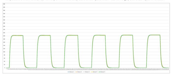
The test results show that the repeatability error range is <2ppm (500ppm ± 1% of full scale is the normal range);
