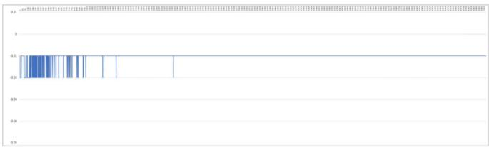
Test result: 12 hours clean air test, zero drift <0.02ppm (0-0.02ppm is the normal zero fluctuation range);
