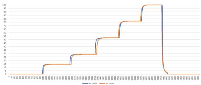
Test result: 100ppm full scale linearity error <± 5%;
