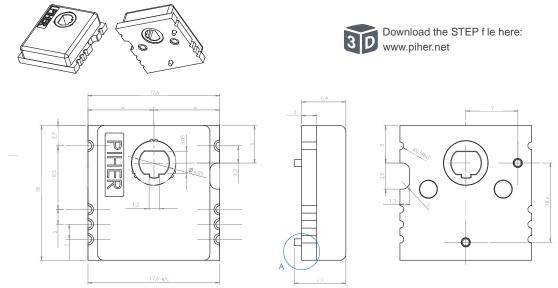
Rotor is shown at zero position. Sensor is delivered at random position
