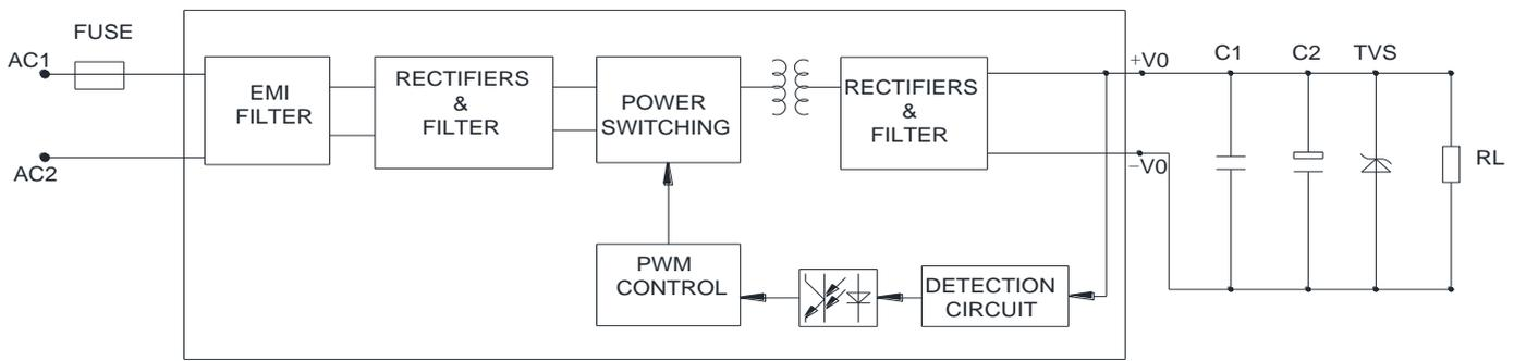
Note; The power supply is considered a component which will be installed into a final equipment. The final equipment must be re-confirmed that it still meet EMC directives.
