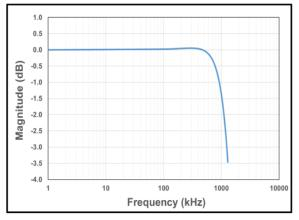
Figure 7: CT430 Bandwidth with C<sub>FILTER</sub> = 1.0 pF
