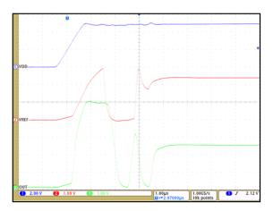
Figure 5: CT430 Startup Waveforms for V<sub>OQ</sub> = 2.50 V (AC Current)
