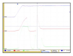
Figure 4: CT430 Startup Waveforms for V<sub>OQ</sub> = 0.50 V (DC Current)
