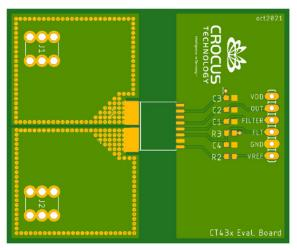
Figure 23: Recommended PCB Layout (Top Layer) for the 20 A to 65 A variants of the CT430
