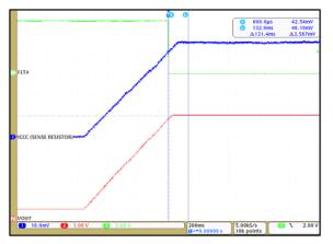
Figure 11: CT430 OCD enabled at 110% of 50  $\rm A_{DC}$  and  $\rm \overline{FLT}$  is Low
