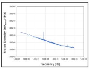
Figure 6: Noise Density vs. Frequency
