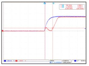
Figure 10: CT430 Propagation Delay;  $I_P = 50 A_{PK}$ and  $C_L = 100 \text{ pF}$  (Blue =  $I_{CCC}$ , Red =  $V_{OUT}$ )
