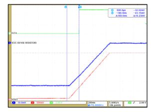
Figure 16: CT430 OCD disabled at –90% of –50  $A_{PK}$  and  $\overline{FLT}$  is High
