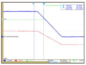
Figure 14: CT430 OCD disabled at 90% of 50  $A_{PK}$  and  $\overline{FLT}$  is High
