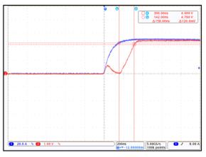
Figure 8: CT430 Response Time;  $I_P = 50 A_{PK}$ and  $C_L = 100 pF$  (Blue =  $I_{CCC}$ , Red =  $V_{OUT}$ )
