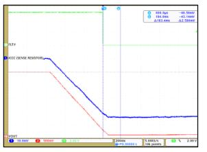
Figure 15: CT430 OCD enabled at –110% of –50  $A_{PK}$  and  $\overline{FLT}$  is Low
