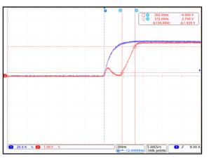
Figure 9: CT430 Rise Time;  $I_P = 50 A_{PK}$  and CL = 100 pF (Blue =  $I_{CCC}$ , Red =  $V_{OUT}$ )
