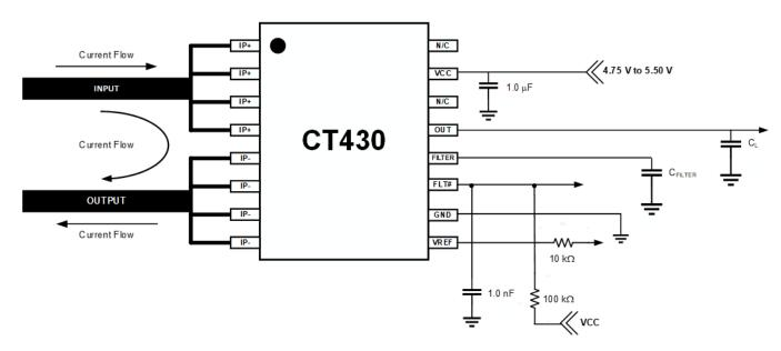
Figure 22: CT430 Application Block Diagram
