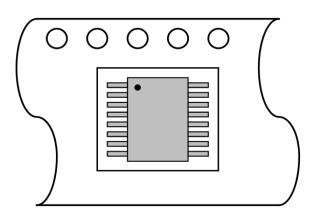
Figure 29: SOICW-16 Orientation in Tape Pocket
