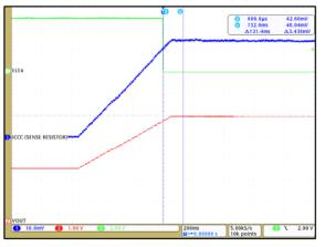
Figure 13: CT430 OCD enabled at 110% of 50  $A_{PK}$  and  $\overline{FLT}$  is Low
