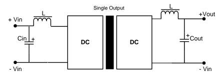
It is not recommended to connect any external capacitor in the application field when output loading is less than 0.5 watt.
