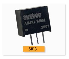
Aimtec's AMSR1-Z is a 1A Switching Regulator which is designed to be a plug and play alternative to the traditional 78xx series three-terminal linear regulators. The series features an ultra-wide input voltage range of 4.6-36V, 1.5mA ultra-low no load input current, continuous short-circuit protection, low ripple noise (max.: up to 50mV) and much more.
