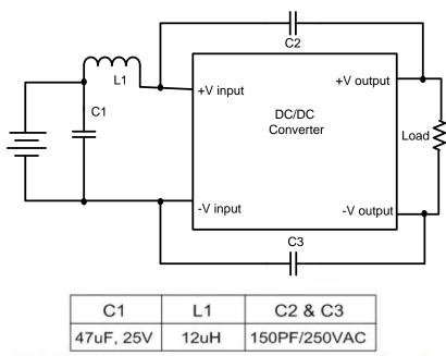
C2 & C3 : Y5P Safety Standard Recognized Ceramic Capacitors foot distance 10mm
