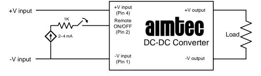
Note: Input current(2~4mA) via 1K $\Omega$  to Pin2, converter OFF. Open or high impedance, converter ON.
