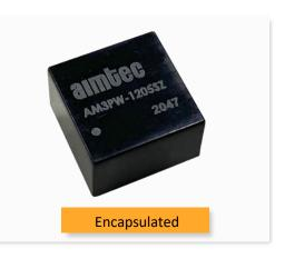
The AM3PW-Z is a DC/DC converter that offers greater cost effectiveness due to material normalization and production automation also leading to improved reliability and performance. Offering an ultra-wide 4:1 input voltage range of 4.5 to 75VDC and an output voltage range from 3.3 to 15V &  $\pm$ 5 to  $\pm$ 15, this series will offer many benefits to your new system design.
