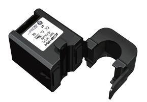
Split-core current transducer for the electronic measurement of AC waveform currents, with galvanic isolation between the primary circuit (power) and the secondary circuit(measurement). 0-5V DC, output proportional to the RMS value of the primary current.
