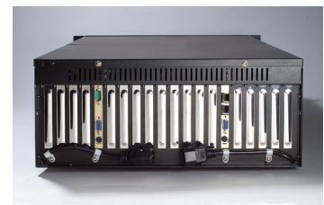
Dual AC power cords for 460W / 570W / 810W redundant power supply
