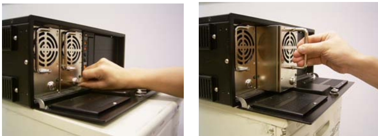
Figure 3.4: Unlock and replace the 460W power supply module
