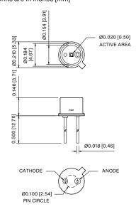
Note: Lead soldering temperature (1/16 inches from case)  $260^{\circ}\text{C}$  for 3 sec.
