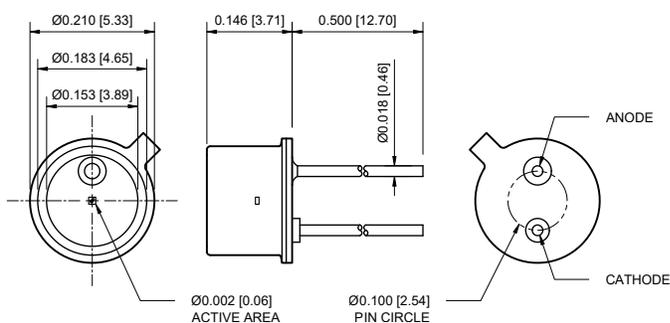
Note: Lead soldering temperature (1/16 inches from case) 260 $^\circ\text{C}$  for 3 sec.
